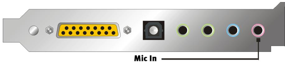
You can control the sensitivity in the ControlPanel for XFire 1024. There is also a switch for the installed pre-amplification of the microphone input. This knob - labeled “Boost” amplifies the signal by +20dB, but also causes more noise.
