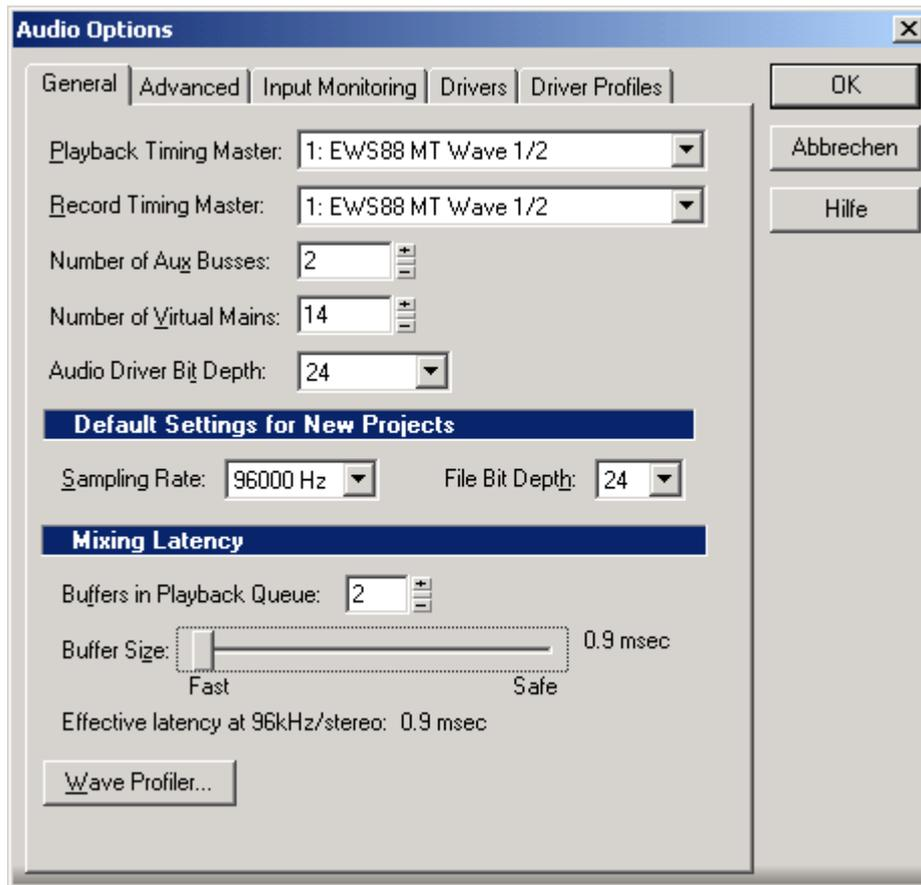
Using the Buffer Size controller you can adjust the latency. Additionally using a smaller value in the field “Buffers in Playback Queue” will further optimize the latency time.
