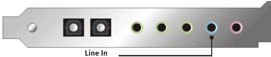
The port format is mini-jack (3,5mm stereo) which can, for example, be connected to the TAPE deck RECORD output on your amplifier or with the AUX SEND port of a mixer. The input sensitivity can be regulated, and is so designed that by a signal level of about  $2V_{RMS}$  maximal level is reached when the appropriate recording slider in the Control Panel is set to 0 dB.
