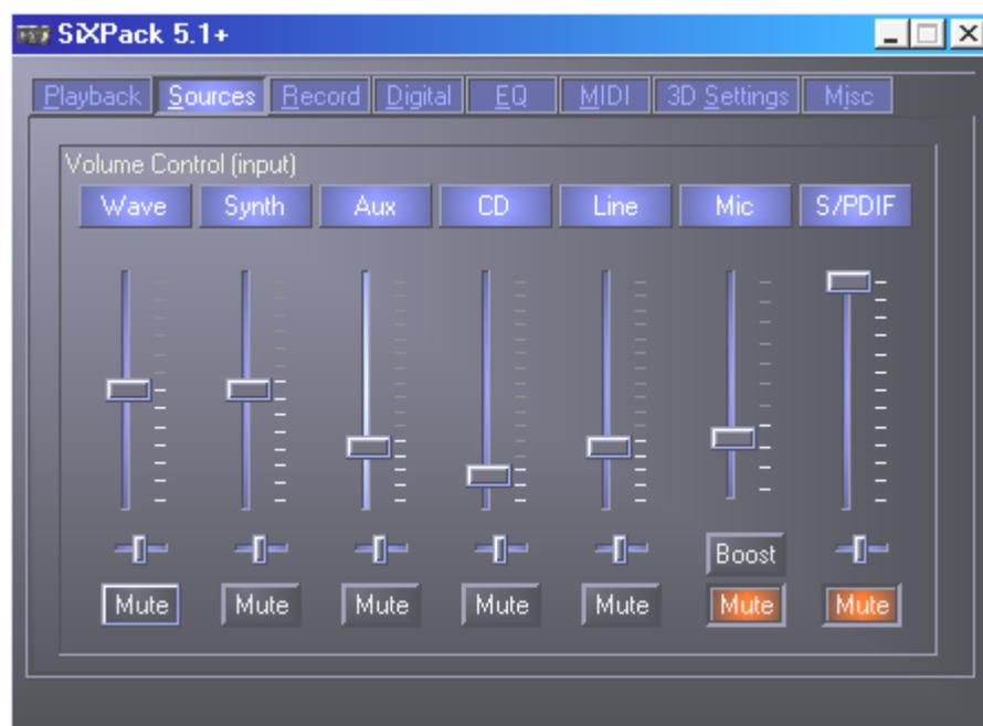
All sources can be muted immediately by clicking on the MUTE option. These sources will still be recorded when chosen for recording, as we are in the source - and not the recording menu. The stereo positioning can be adjusted using the panorama controller located under the volume sliders.
