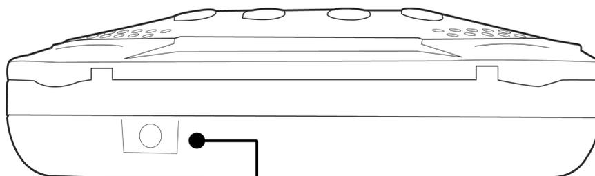
*Plug for the electricity adaptor cable (DC 5 V/600 mA).*
