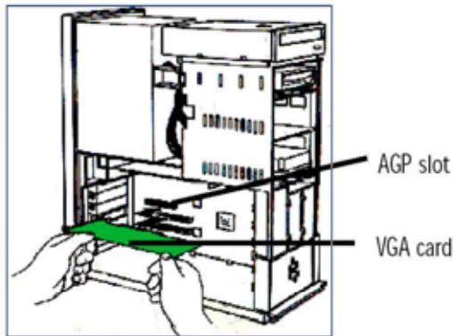
3. Remove the old graphics board if present. First, remove the screw holding the slot plate of the card to the case. Grasp the card by the edges and carefully pull it out of its slot. Next, carefully insert your TerraTec Mystify 440 into a free AGP slot and gently press it into the slot until completely seated.
