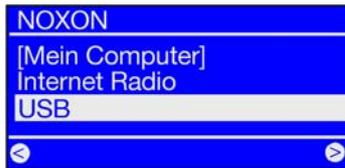
An entry for the USB storage media will appear in the main folder of the NOXON whenever a compatible USB storage device is connected. Selecting this entry will display a selection of compatible partitions. If only one is available, “Volume 1” is all that will be shown. Once you have made your selection, the folder structure will be displayed 1:1. Next, use the usual navigation to select and play a track.
