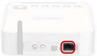
Two LEDs near the port show the status of the **link**: **orange** indicates a live connection to the network junction (“node”); network **traffic** is signaled by a **green** LED (usually flickering).
