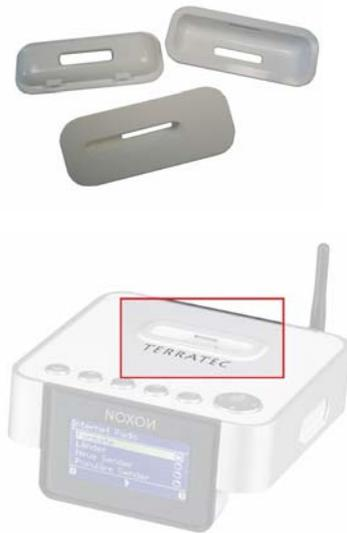
For proud iPod owners, there's a recess on the top of the device with an iPod docking station. To use it, remove the protective cover. This port allows you to play back and charge your iPod quickly and easily. For playback, the iPod is controlled directly from the NOXON main menu—of course, you can make a selection and operate it by remote control as well.
