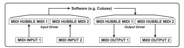
Operation in Windows: MIDI Input/Output routing with driver open
