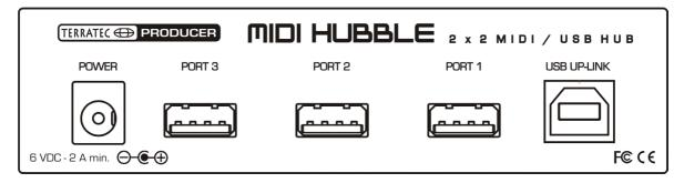
The optional AC adaptor can be connected to the **power socket** on the rear panel. This socket is intended solely for use with the TerraTec AC adapter (article number 200067) which is available as an optional extra. In most cases, however, the MIDI HUBBLE can be used without an AC adapter (bus powered mode). Please read the power supply notes starting on page 5.
