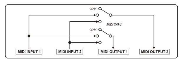
Operation in Windows: MIDI Input/Output routing with driver closed
