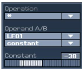
The ARITHMETIC section is really something special. You can use it to link two operands using logical functions. The results are available as modulation sources. A simple example is inverting an LFO waveform. To do so, multiply the LFO by a negative constant value. You can then select the inverted waveform as the source under "Arithmetic 1".
