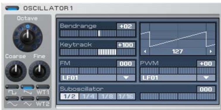
Oscillators 1+2 are identical except for a few details. You can determine the basic pitch using Octave, Coarse and Fine. The six buttons for the waveform are located below. For the waveforms Pulse, WT1 and WT2, you can change the pulse width
