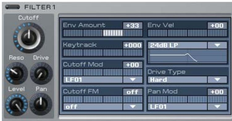
Filters 1+2 have an identical layout and, when not in use, can be disabled using the button next to the label in order to conserve CPU resources. The filters have an especially wide range of functions and feature ten different filter type models.
