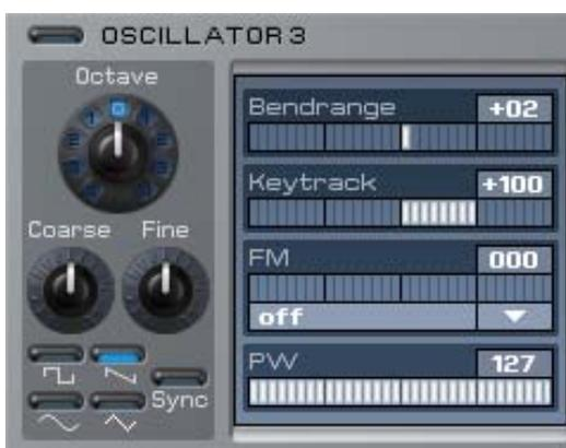
Oscillator 3 does not have any wavetable waveforms, but can be synchronized with oscillator 2. You can set the pulse width of the pulse waveform under PW and modulate it in the modulation matrix on the MATRIX screen. If Sync is activated, oscillator 3 is synchronized with oscillator 2. Experiment with envelope curves or LFOs in oscillator 2 in order to obtain typical sync sounds. To do so, oscillator 3 must be enabled and its level set to > 0 in the mixer.
