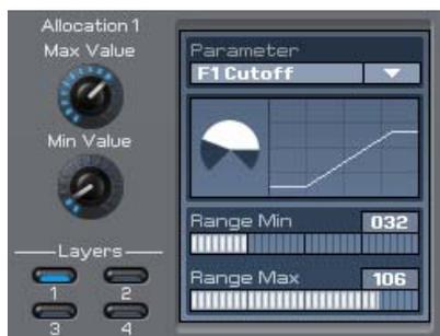
For each parameter, you can now define in which knob range it is affected by the MACRO controller and how strongly it is affected. Here, the Max and Min values define the maximum and minimum values that the parameter can have. It is also possible to create negative directions. Range Min and Range Max define the turning range of the knob in which the parameter is changed.
