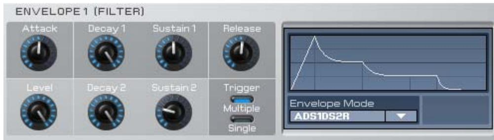
As the name implies, you can edit the four envelope curves and the three LFOs in detail on the ENV/LFO screen. Each of the four envelope curves offers the following modes:
