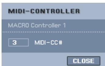
enter a number directly using the computer keyboard or move an operating element on your hardware controller. If the controller outputs a MIDI CC, the number automatically appears in the allocation window (learn function). Click OK to accept the change. If the same MIDI CC has previously been
