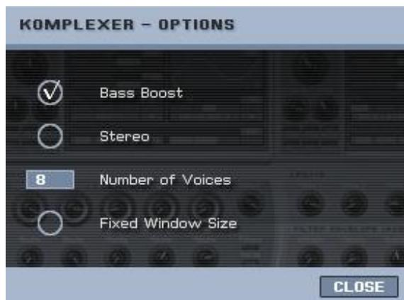
**Fixed Window Size** – The KOMPLEXER VST keyboard window is smaller than other windows. Some audio programs do not support different window sizes within one plugin. You can select this option to define a fixed window size so that KOMPLEXER VST always appears in full view.
