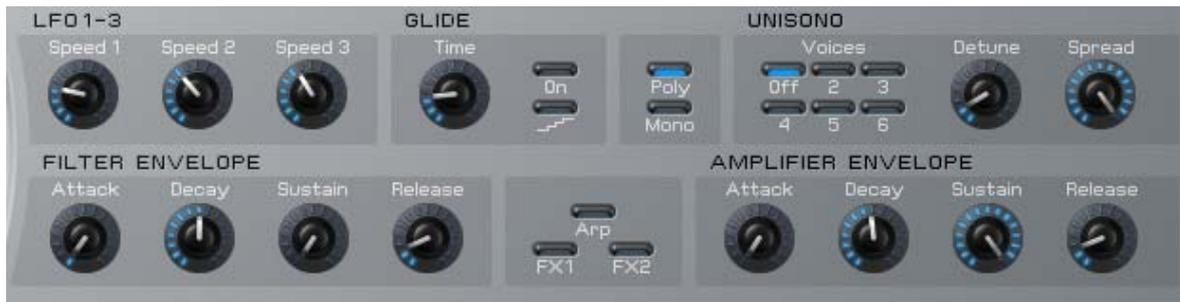
**LFO 1-3** - Control the speed of the LFOs (Low Frequency Oscillator); the same parameters are also present on the ENV/LFO screen.
