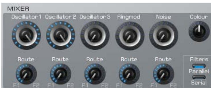
The MIXER mixes together the oscillator, the ring modulator and noise. Use the Route knobs to mix the respective source to Filter 1 and/or Filter 2. The Color parameter changes the color of the noise from brown to white (middle position) to pink.
