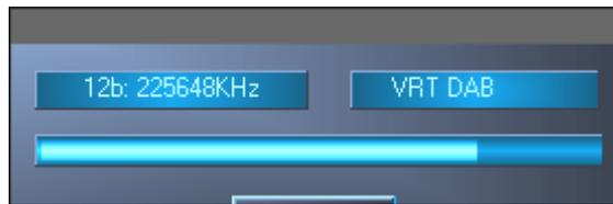
Upon reception, quality is symbolically represented by the blue bar (**receiving signal strength**) above the station selection. The station selection, as known from the unit itself, contains ensemble name and station name. Clicking on the bar to the right of the station display toggles between stations of an ensemble.
