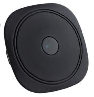
The TERRATEC CONNECT BT makes music wireless. The small adapter is easily plugged on the 3.5 mm jack connection of the hi-fi system, of the mobile loudspeakers or another output device and the transfer of music from the Smartphone, Tablet and similar devices can be performed wireless.
